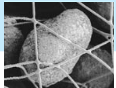
Gas contaminants must pass through tortuous pathways coming in intimate contact with the carbon. The fibers anchor themselves to the carbon using only 1% of the carbon’s surface helping to maximize the contaminant’s exposure.
